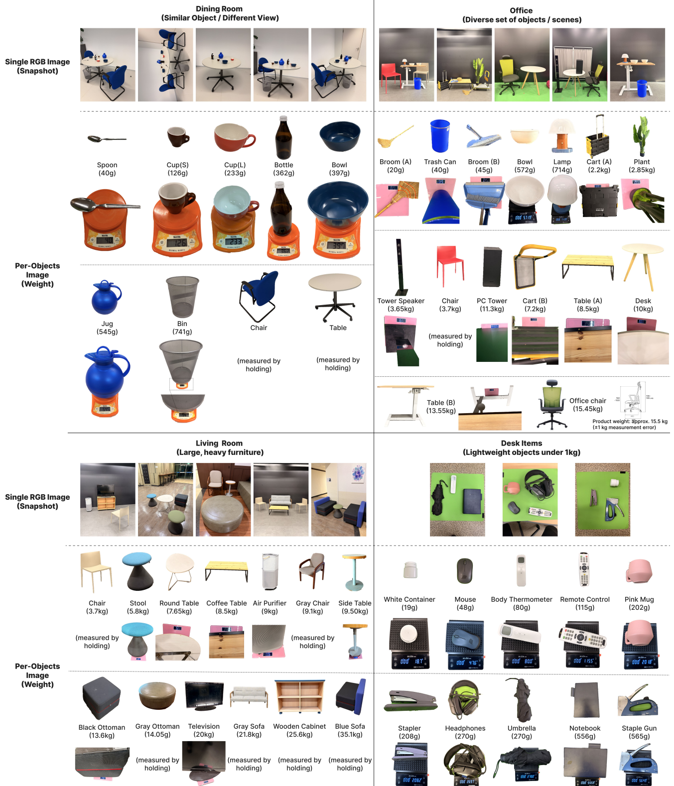
Figure 1: Per-scene dataset visualization. For each scene, we show (top) single RGB images captured from multiple viewpoints, and (bottom) per-object images with ground-truth mass values measured using a digital scale. For large objects (Chair, Table), mass was measured via a human subtraction method and scale photographs are omitted accordingly.
